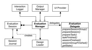
Figure 1: **High-level structure of evaluation library.** The EvaluationManager controls the evaluation. The abstract EvaluationDelegate needs to be implemented to connect the library to the visualization artifact.
