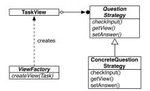
Figure 4: **ViewFactory.** Creates a view for a given task, whereas the QuestionStrategies provide a subview, set the answers, and check for sufficient input for each question.
