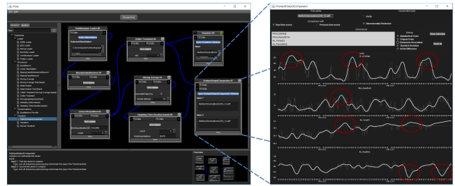
Figure 10: Final pipeline applied on the longitudinal climate data set. The analyst has put two “visual sensors” to the output of the OutlierTreatment and Sampling routine to facilitate the visual comparison of different branches. Right: the comparison reveals that the outlier routine (gray) would have cut considerable parts of the peaks, which have been preserved with the final branch (white).
