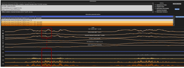
Figure 7: Assessment of the effect of a sampling routine to six selected dimensions ( T_R , T_P , T_D ). The Quartile Trend Chart at the bottom depicts the uncertainty for every parameterization (aggregated over dimensions, cf. Table 2). The blue parameterization (5 minute kernel) almost introduces no uncertainty, in contrast to considerable changes caused by the orange kernel (40 minutes) ( T_U ).
