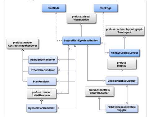
The architecture of this visualization looks nearly the same as the detail visualization in the O+D mode, the only difference is the usage of the *FishEyeLogicalLayout* for element positioning and the *PlanRenderer* instead the standard prefuse LabelRenderer. This is necessary because in this mode, a (sub)plan cannot only be expanded or selected, but also opened.
