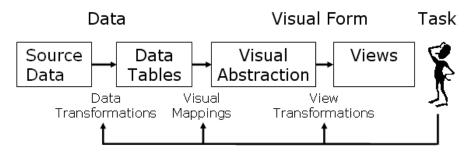
The next figure below illustrates how the different classes of the prefuse toolkit implement the reference model:
