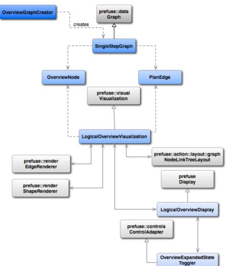
Since this visualization only displays the plantree without other elements such as ask, if-then-else assignments,.., a OverviewGraphCreator is responsible for the creation of the SingleStepGraph. This visualization is much simpler than the detailed visualization, so the standard prefuse renderers and layout-algorithm are adequate. The OverviewDisplay also has a ExpandedStateToggler that recognises clicks on the nodes.
