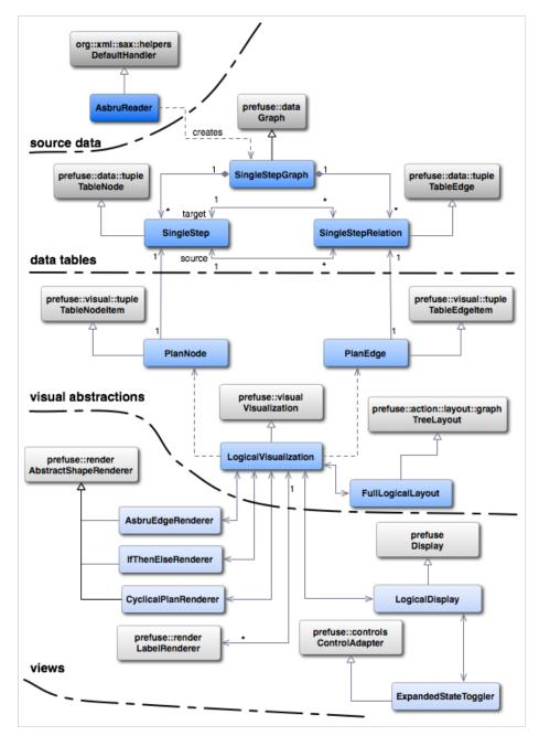
The class AsbruReader, which is a XML Parser for Asbru files, creates a SingleStepGraph consisting of SingleSteps connected with SingleStepRelations. The visual representations of this graph is a VisualGraph consisting of the visual representations of SingleSteps and SingleStepRelations: PlanNodes and PlanEdges. These visual elements get visualized by the LogicalVisualization, applying a FullLogicalLayout on them, does some coloring and is responsible for the animations.
